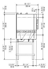
CWII Cold Water inlet 1 CWI2 Cold Water Inlet 2 ΕI Electrical inlet (power) Gas connection
